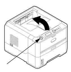
**2.** Holding it by its top centre, lift the used image drum and toner cartridge, out of the printer.
